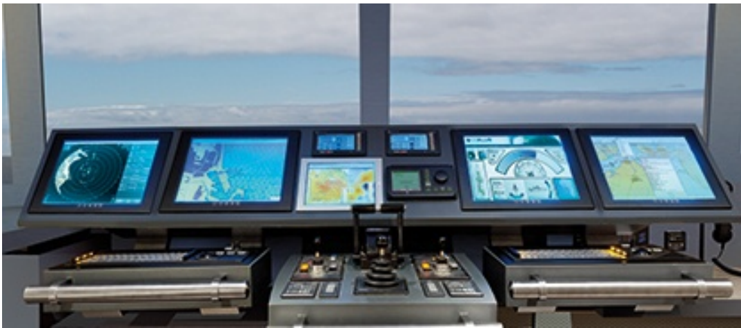
Figure 5.2 - Ship's Control Bridge from iXblue [22]
