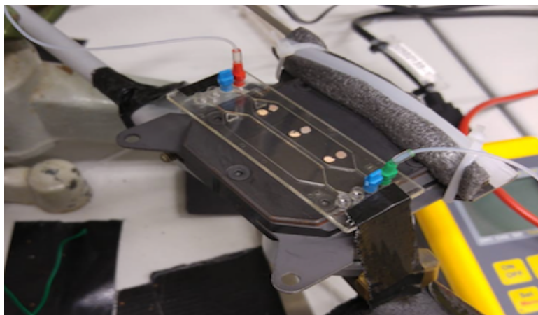
Figure 11. Picture of the pumping set-up without the isolation cover.
