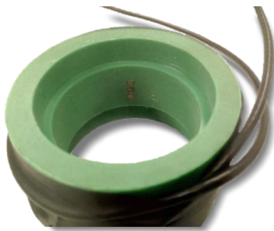
Figure 5. View of the custom manufacturing port of the conductance probes.
