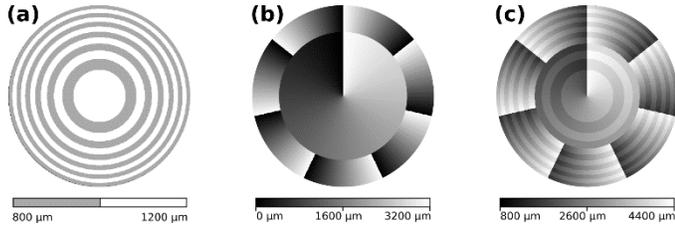
Fig. 1. Design of a multiplexed THz vortex lens. a) Base FZP using (1) with  $p = 1/6$ , b) Multiplexed vortex SPP with topological charges inner part and outer part. c) Composite vortex lens as the superposition of a) and b). Gray levels represent the lens thickness.
