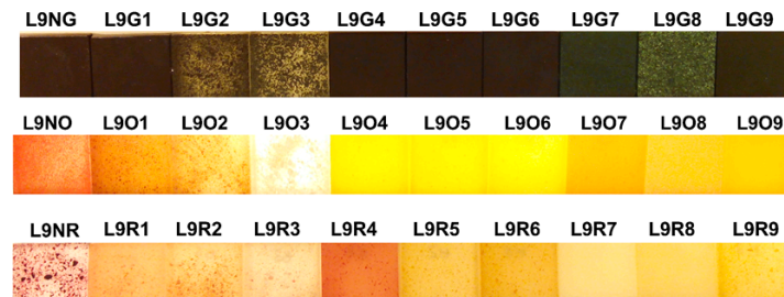
Figure 10. Maximum concentrated samples (10%) for the composite materials from the nano-pigments made by the L9 experiments with three natural dyes: NG, NO, and NR.
