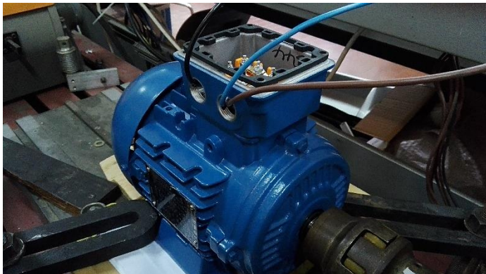
Fig. 5 – Induction machine used for experimental tests.
