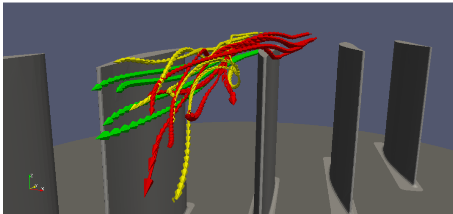
Figure 5.13: Flow characteristic patterns in a compressor cascade. View from lateral right side ( i=10^\circ , Re=27.422 , h=4\% )
