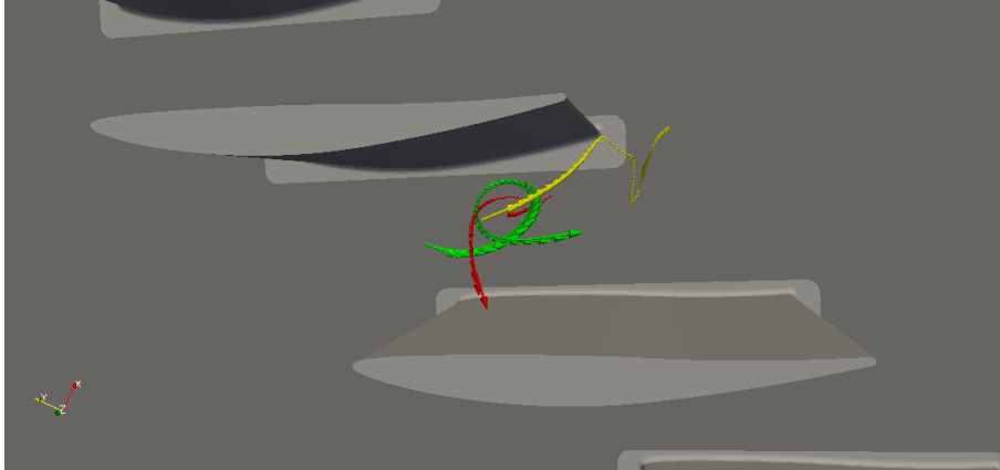
Figure 5.35: Flow unstable patterns in a compressor cascade. View from top ( i=19^\circ , Re=30.023 , h=4\% )
