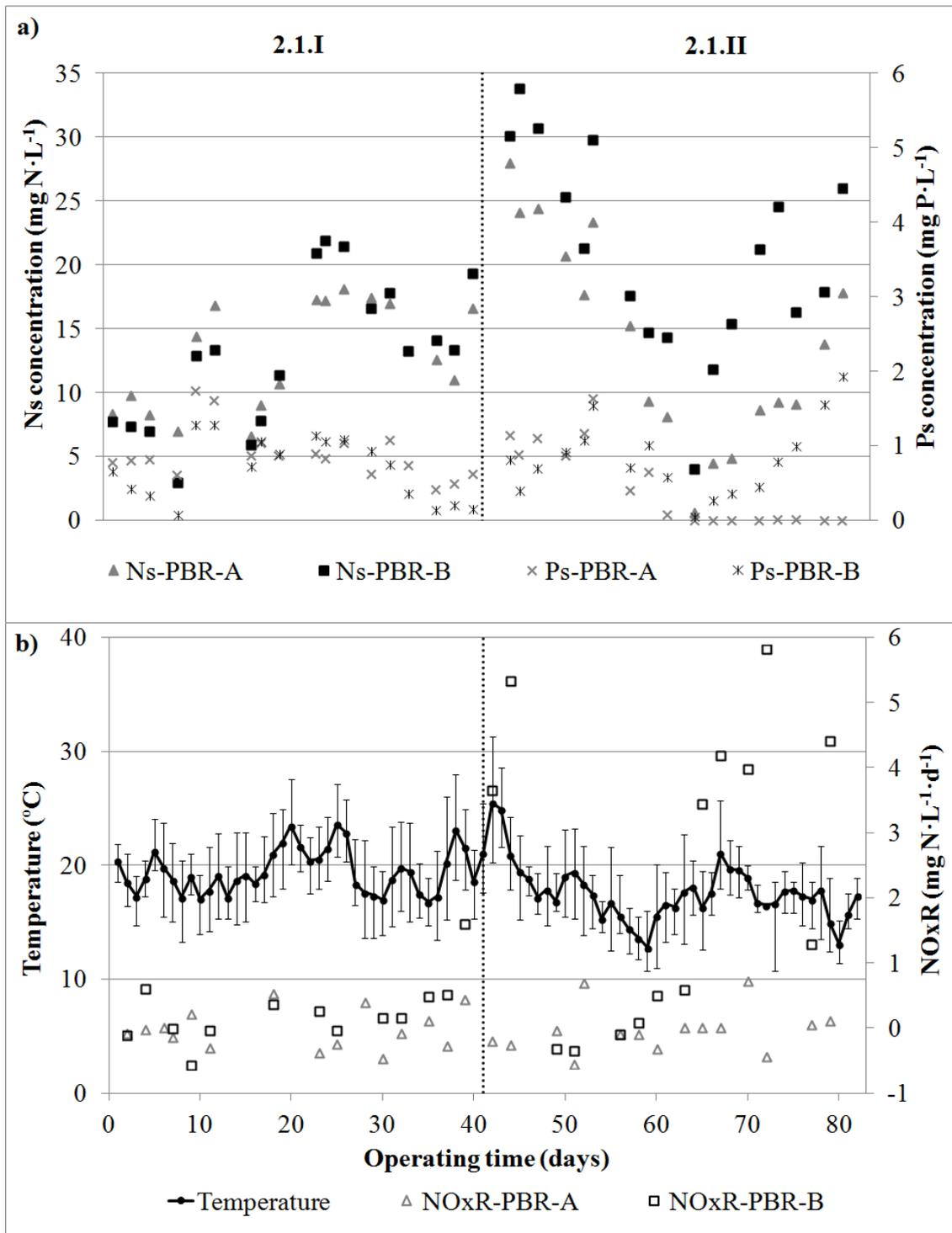
Figure 4. Evolution during experiment 2.1 in PBR-A (inhibited nitrification) and PBR-B (free nitrification) of: a) nitrogen (Ns), and phosphorus (Ps) concentrations; b) temperature and nitrification rate (NOxR).
