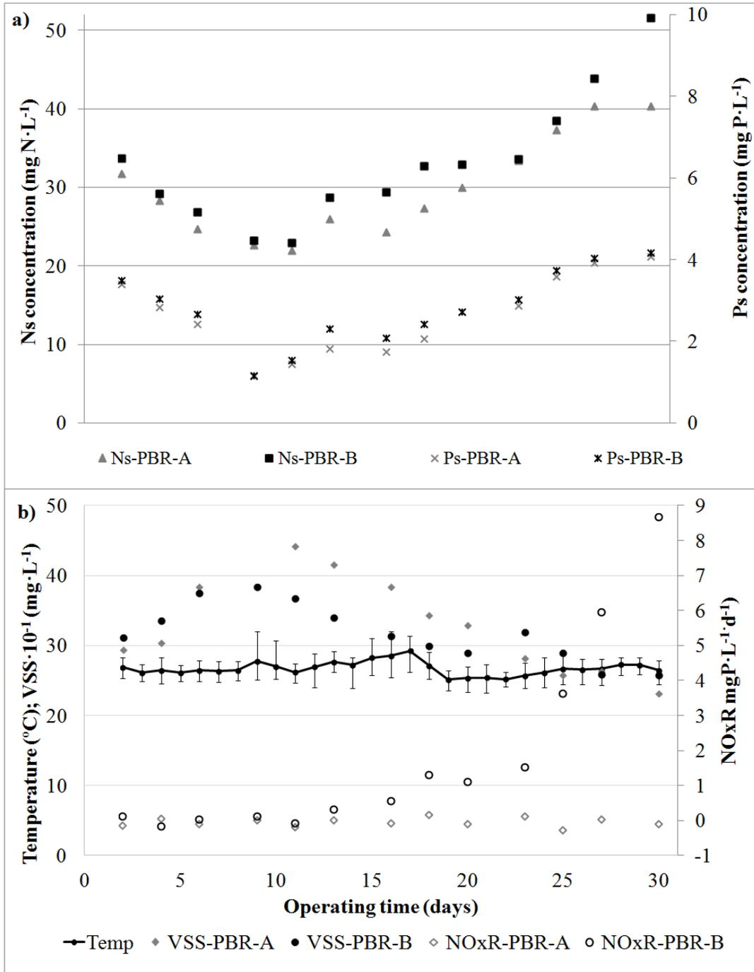
Figure 5. Evolution during experiment 2.2 in PBR-A (inhibited nitrification) and PBR-B (free nitrification) of: a) nitrogen (Ns), and phosphorus (Ps) concentrations; b) temperature, volatile suspended solids (VSS) concentration and nitrification rate (NOxR).
