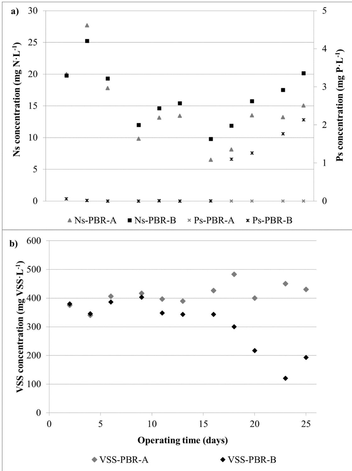
Figure 3. Evolution during Experiment 1.4 in PBR-A and PBR-B of: a) nitrogen (Ns) and phosphorus (Ps) concentrations; b) volatile suspended solids (VSS) concentration.
