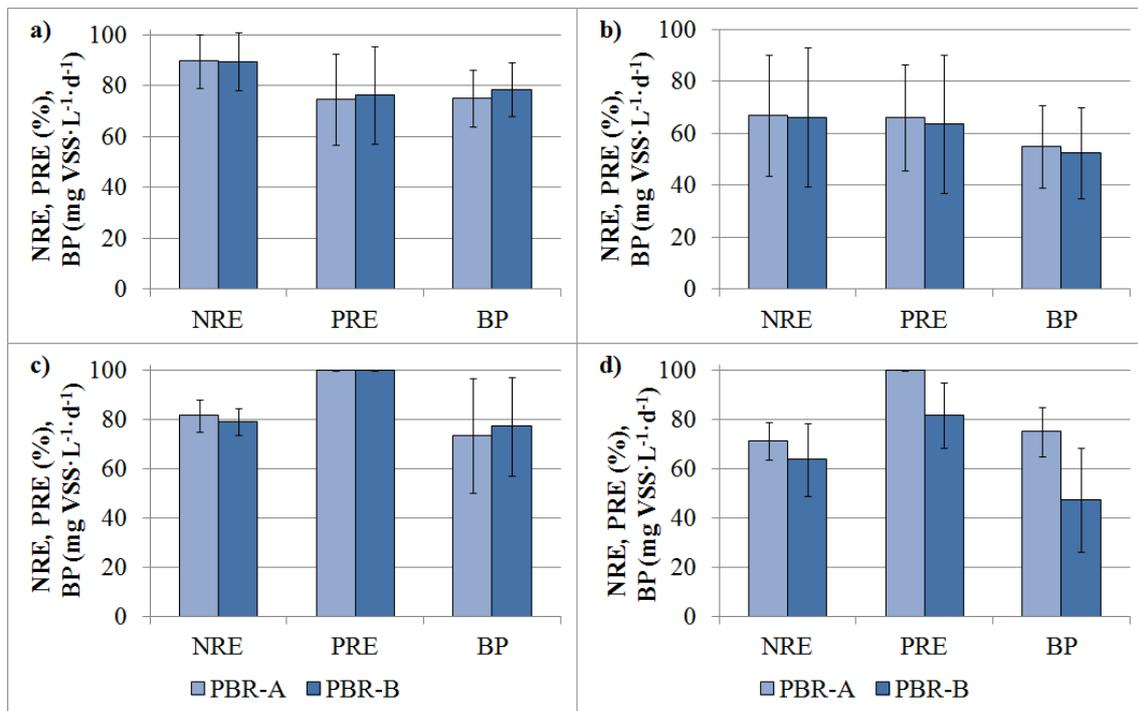
Figure 1. Effect of temperature in biomass productivity and nutrient recovery. Mean values of NRE, PRE and productivity. PBR-A: temperature controlled at around 25 °C; PBR-B: free temperature. a) Experiment 1.1 (autumn); b) Experiment 1.2 (winter); c) Experiment 1.3 (spring); d) Experiment 1.4 (summer).
