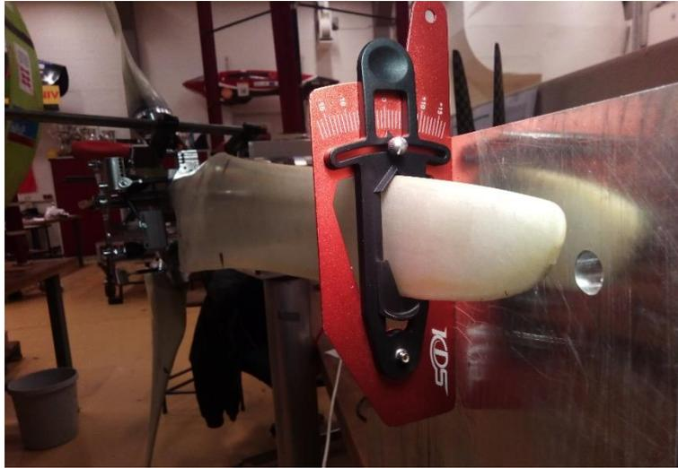
Figure 11. Aligning the blade with respect to the rotor plane.
