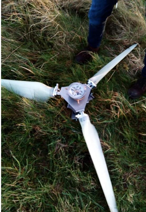
Figure 50. SWT rotor after fatigue break
