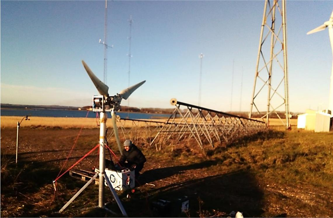
Figure 46. Arrangement in the Risø test field. The DTU SWT is shown in first plane, fixed to the ground with ropes and stakes. Behind, the electronic devices for live monitoring and controlling the SWT. The anemometer can be seen in the left side of the picture.
