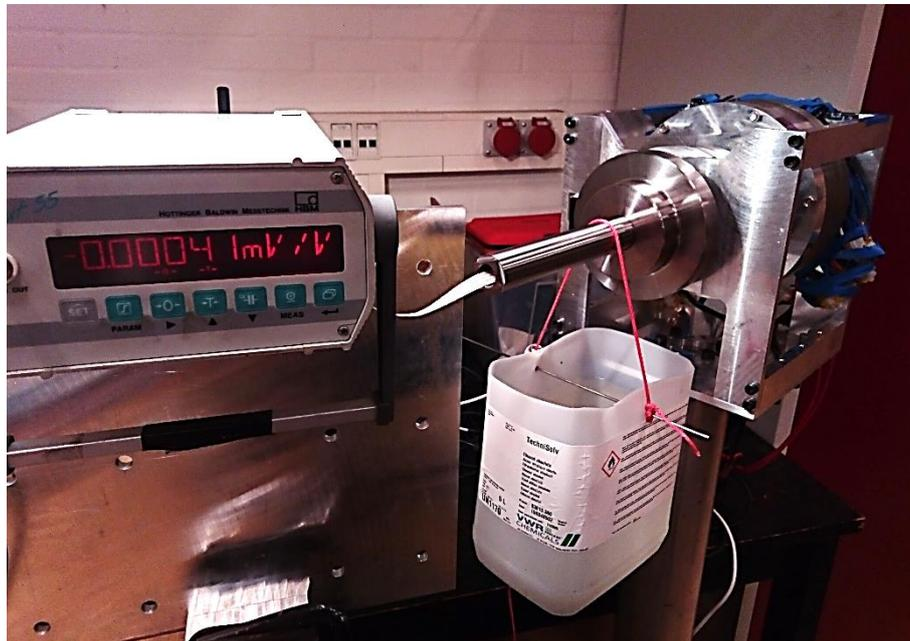
Figure 78. Crosstalk measurement. In this figure can also be seen the utilized portable amplifier SCOUT55, and the water container.
