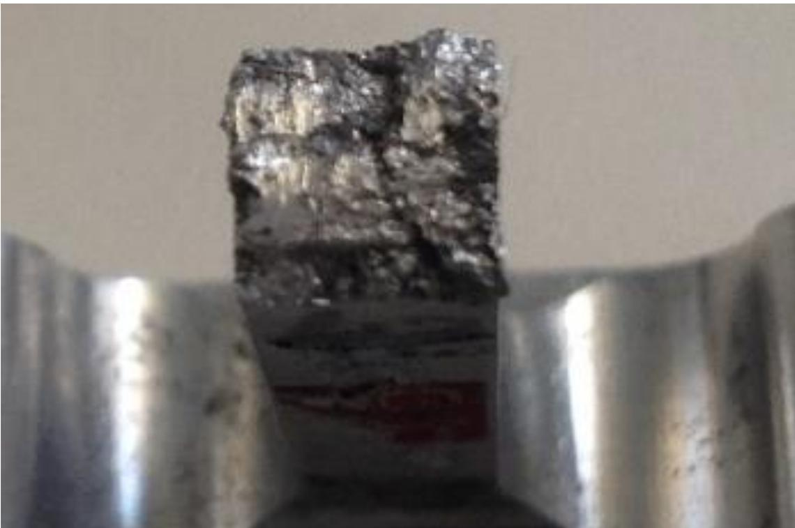
Figure 53. Sudden fragile fracture detail.
