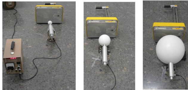
Figure 6. ^{241}\text{Am} -Be neutron source measuring with the BSS system
