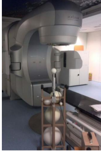
Figure 2. BSS detector measuring neutrons in a radiotherapy Linac room.
