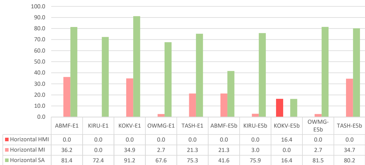
Figure 4.12 – Campaign horizontal integrity results on Date #1 for GALILEO-OS.
