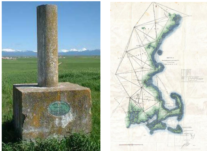
Figure 2.2 – Geodetic monument and geodetic network example. Source: Wikipedia.org.
