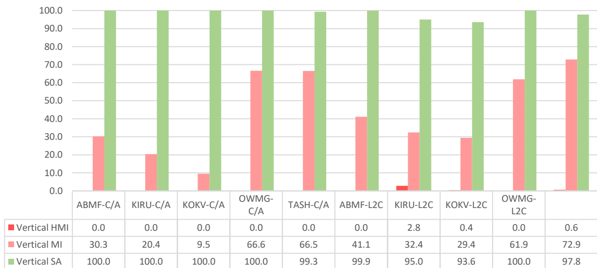
Figure 4.15 – Campaign vertical integrity results on Date #2 for GPS-SPS.
