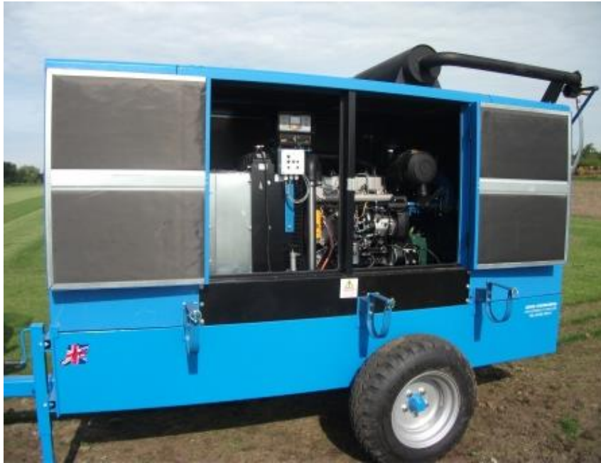
Figure 10: Jones Engineering's Pump (open)
