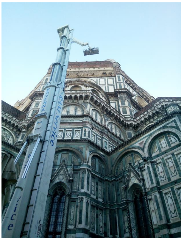
Fig. 3. November 2018, the photogrammetry campaign of the Florentine Cathedral: northern absis (Source: own's, the author).
