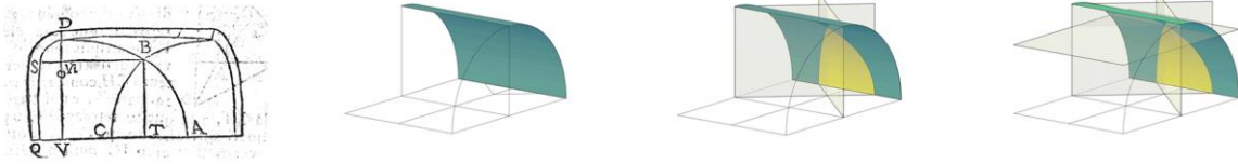
Fig. 12. Guarini, surface to be subtracted for inserting a lunette. (Source: Guarini, 1674, Proposition 16. Modelling: author).
