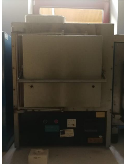
Figure 3. 2. Oven employed ( Termolab ) for the curing cycle
