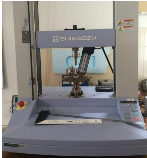
Figure 3. 8. Universal testing machine ( Shimadzu AGS-X )
