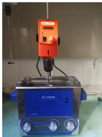
Figure 3. 3. Ultrasonic machine ( GT Sonic ) and mixer ( lhx Instruments ) employed
