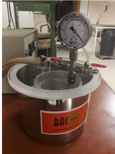
Figure 3. 4. Vacuum chamber employed ( Baco Eng )
