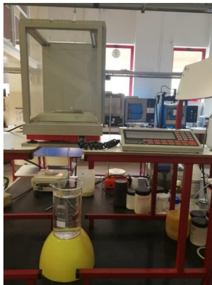
Figure 3. 6. Measurement equipment ( Oertling VA204 ) configuration to measure Suspended Weight
