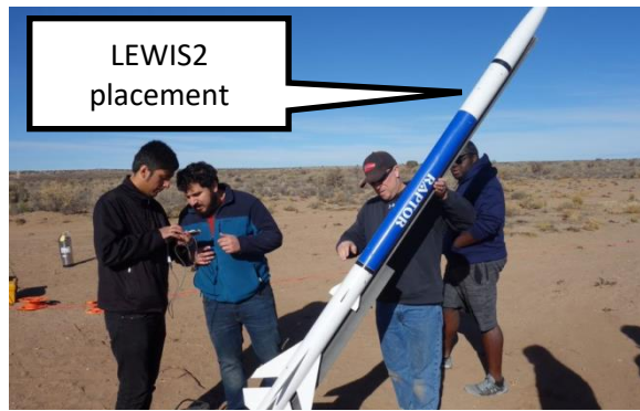
Figure 3-7. Activation of the wireless sensor remotely to record the acceleration and angular velocity.
