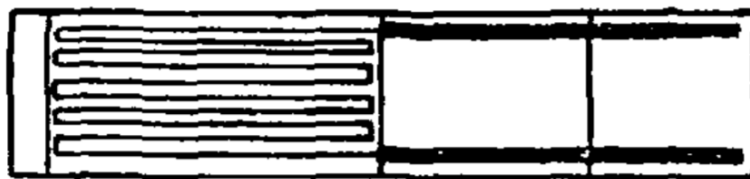
Figure 3.5. Form of a resistance strain gauge [6]
