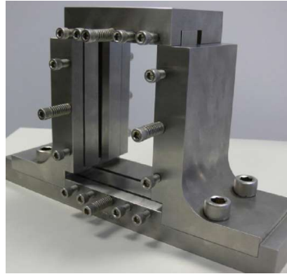
Figure 2. CAI test device from Zwick/Roell GmbH company according to ISO, Airbus, EN [35]
