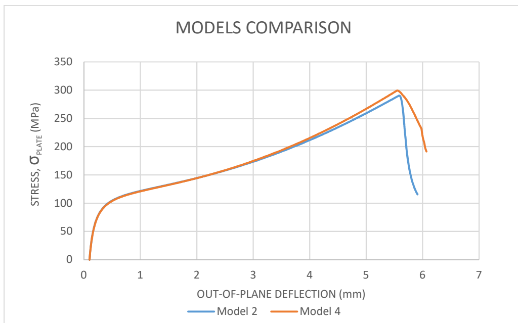
Figure 45. Comparison of the out-of-plane deflection between Model 2 and Model 4
