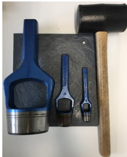
Figure 13. Membrane cutting tools (From left to right, cutting diameters 75, 25 and 13 mm)
