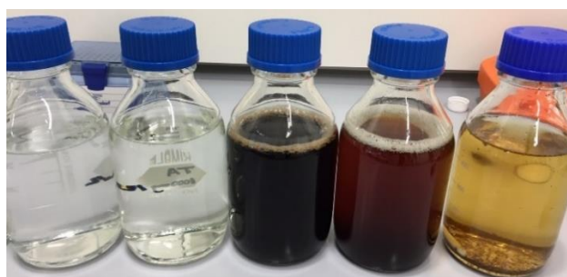
Figure 11. NOM stock solutions (Left to right: Alginate, tannic acid, humic acid, Australian NOM and tea extract)
