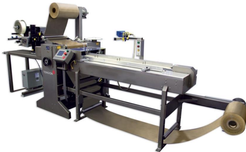
Figure 13. Example of a Cold Seal machine, 9000-18 by Angloscand (“The 9000-18 Cold Seal machine”, 2018)
