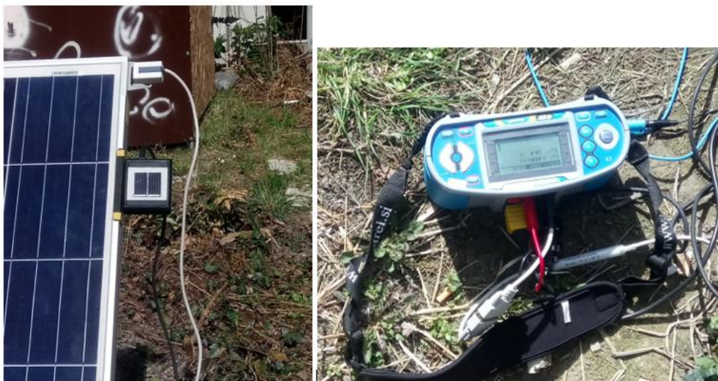
Figure 33 Left: Thermometer (Up), Irradiance Sensor (Down); Right: Solar Analyser
