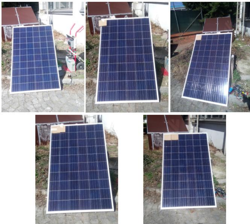
Figure 35 Photovoltaic Module with Different Levels of Shading
