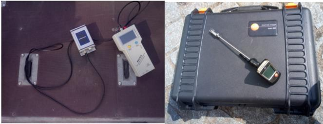
Figure 34 Irradiance Sensor (Left) and Thermometer (Right) used on the Experiment
