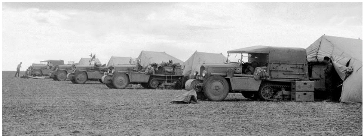
Six P17s took part in the Croisière Jaune, Pamir group. Some sources mention that they were special-built, with chassis from P19, the 6-cylinder sister of P17 of which one was also used in the expedition.
