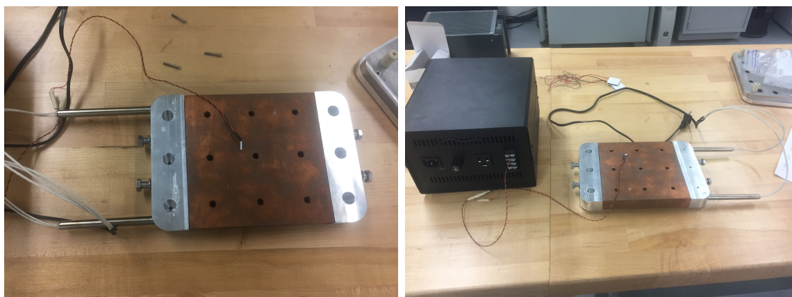
Figure 5.3: Bottom side of the heating plate, without and with the specimen boat.
