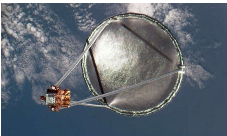
Figure 1.1: Inflatable structure to be sent to the space, where it is going to be subjected to space environmental aspects, being outgassing one of them.
