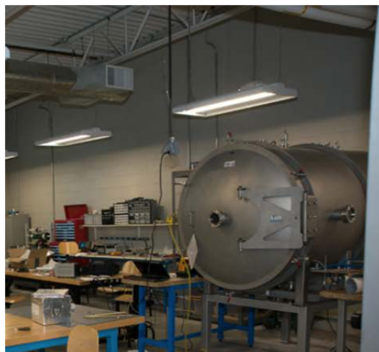
Figure 2.7: Large Vacuum Chamber at ERAU's COAS Astrophysics laboratory.
