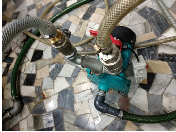
Figure 2.3: Pump with bypass valve configuration
