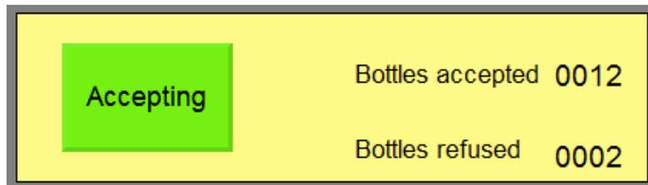
Fig. 27-Quality control section of the HMI showing the results of the quality control process
