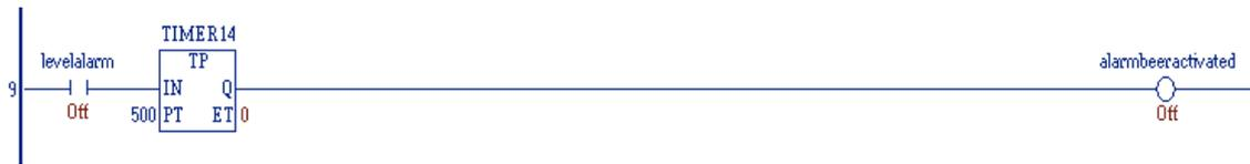
Fig. 19-Ladder program of the filling tank process
