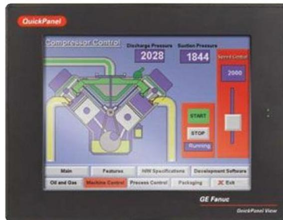
Fig. 1-12" QuickPanel View & QuickPanel Control
