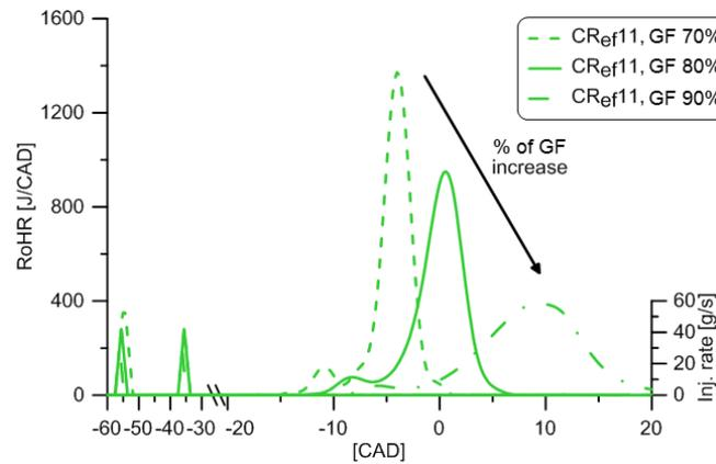
Figure 8: Diesel injection rates and RoHR for different gasoline fractions at a fixed  $CR_{ef}$  of 11:1.
