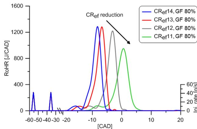
Figure 3: Diesel injection rates and RoHR for different effective compression ratios and fixed GF of 80%.
