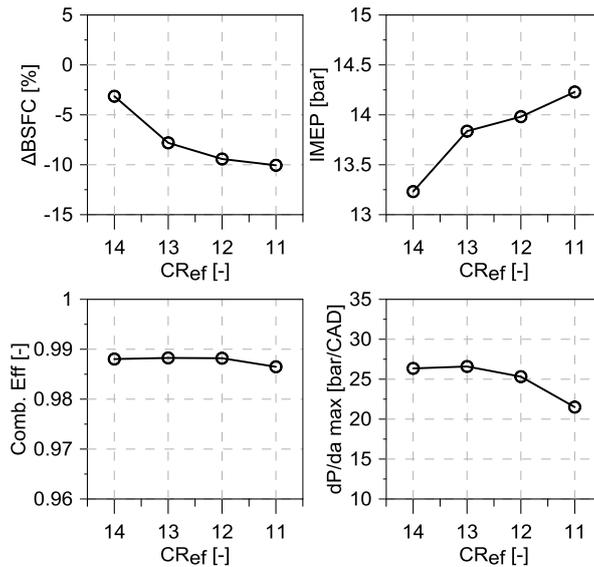
Figure 7: Engine performance as a function of the effective compression ratio at a fixed GF of 80%.
