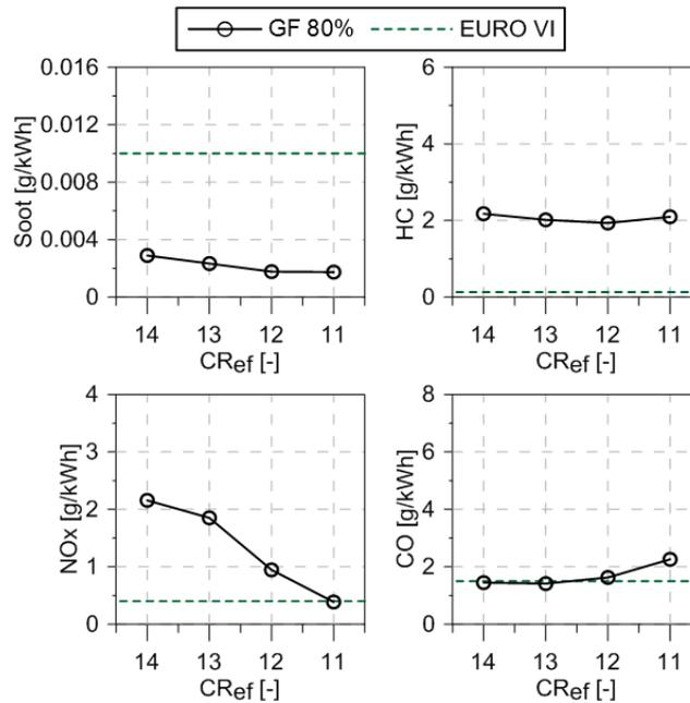
Figure 5: Engine-out emissions as a function of the effective compression ratio at fixed GF of 80%.
