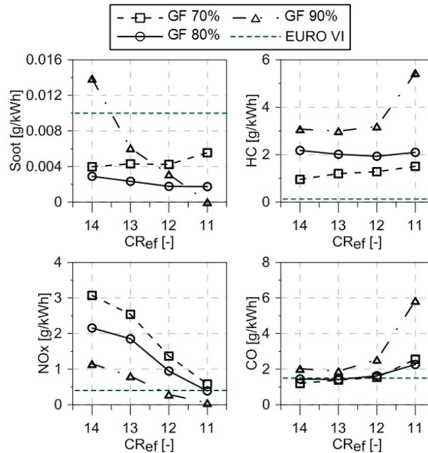
Figure 11: Engine-out emissions as a function of the effective compression ratio for GF 70%, 80%, 90%.
