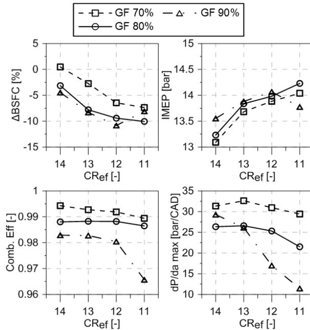
Figure 12: Engine performance as a function of the effective compression ratio for GF 70%, 80%, 90%.
