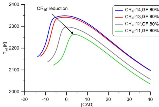
Figure 6: Adiabatic flame temperature for different effective compression ratios at fixed GF of 80%.
