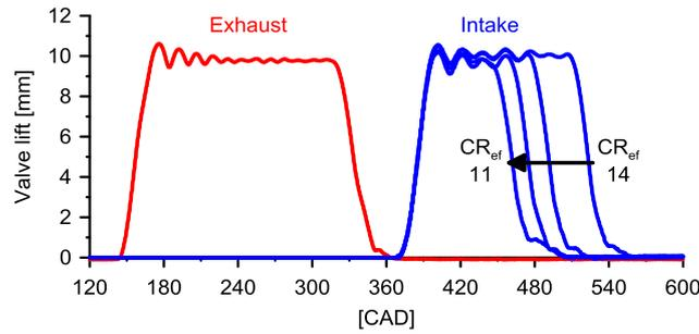
Figure 2. Valve lift profiles for the different Miller cycle.
