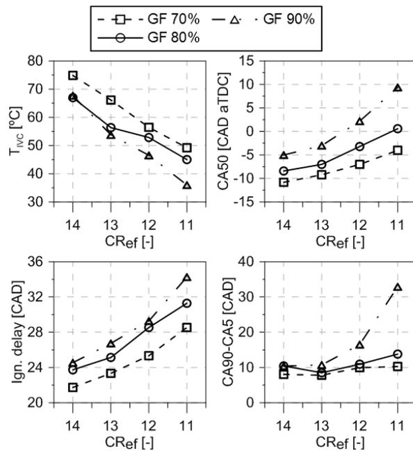
Figure 9: Temperature at IVC, ignition delay, CA50 and combustion duration as a function of the effective compression ratio for GF 70%, 80% and 90%.
