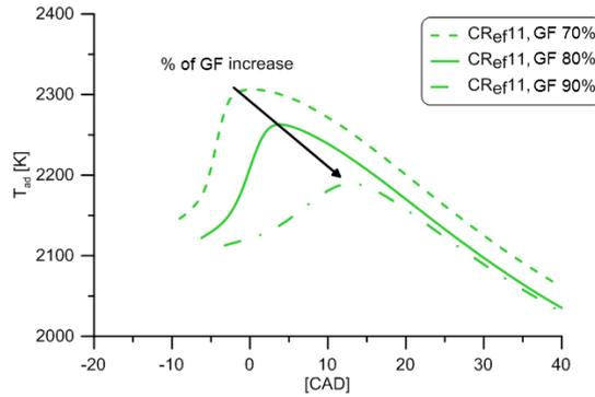
Figure 10: Adiabatic flame temperature for different gasoline fractions at a fixed  $CR_{ef}$  of 11:1.
