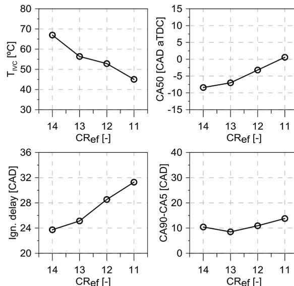
Figure 4: Temperature at IVC, ignition delay, CA50 and combustion duration as a function of the effective compression ratio at fixed GF of 80%.
