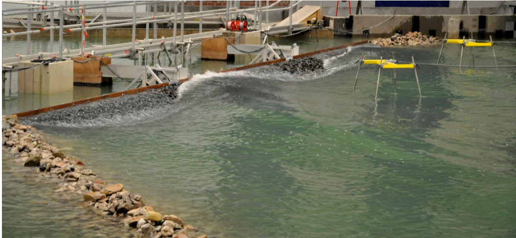
Figure 4. Experimental set-up during a test with oblique waves.
