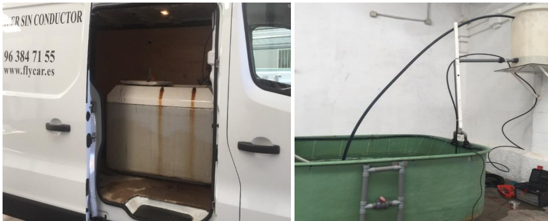
Fig. 48 On the left the fish transport system from the aquaculture center to the UPV laboratory. On the right the acclimatization tank with the oxygenation system.
