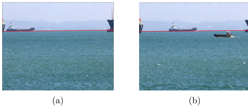
Figure 4.11: Illustration of background subtraction using Method B. (a) Image used to model background. (b) Image used for background removing from model obtained in Image (a).
