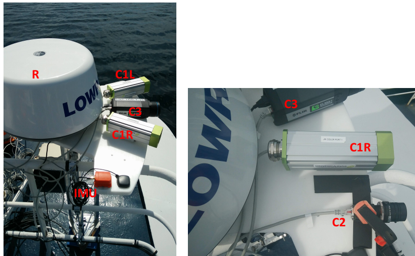
Figure 6.1: Platform used for measurement. In red are annotated different sensors. Radar (R), Inertial Measurement Unit and GPS (IMU), two color cameras (C1L, C1R), one monochrome camera (C2) and FLIR camera (C3).
