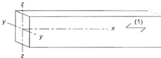
Figure 1. Straight solid timber beam Source: CTE DB SE-M Key: (1) direction of grain
