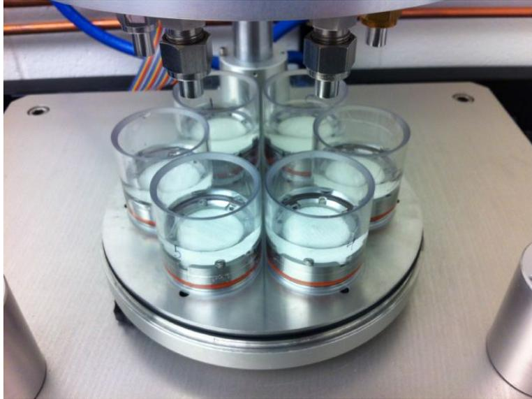
Figure 6: Fabric assemblies installed in Ortho-POD.
