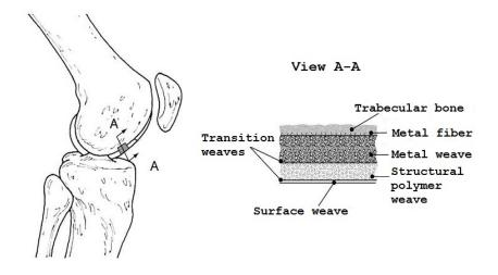
Figure 1: Schematic illustration of the cartilage repair implant, shown on the knee. Some of the design features that can be incorporated into advanced weaving processes are shown on the right.
