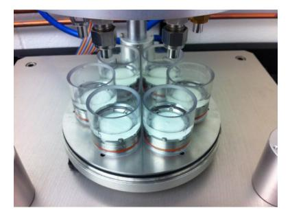
Figure 6: Fabric assemblies installed in Ortho-POD.
