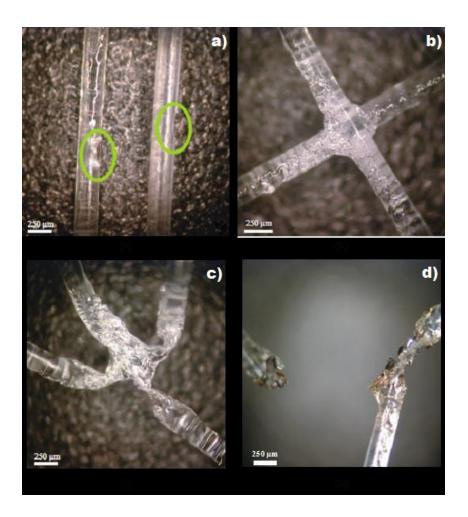
Figure 4: Examples of fiber-fiber welding with a toner. (a) insufficient laser power, leading to poor adhesion; (b) strong weld; (c) and (d) fiber damage resulting in poor weld strength.
