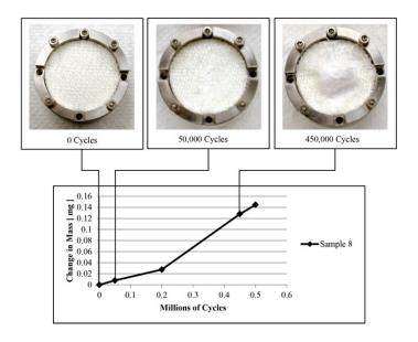
Figure 2: Typical wear results for a conventional woven PET orthogonal woven material. As can be seen, the damage at around 0.5 million cycles is due to fiber pullout and lateral deflection.
