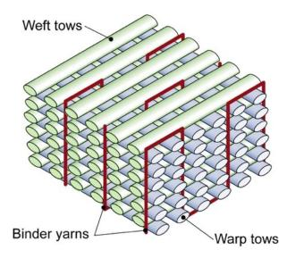
Figure 3: Orthogonal weave, showing weft and warp tow directions and binder yarn. No oblique weaves are considered in this paper.
