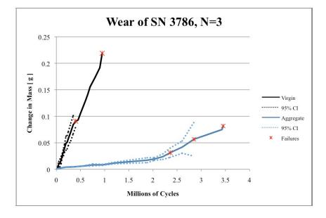
Figure 7: Representative results from wear tests comparing original and welded material. The material is described in Table 1, using three repetitions (N=3).
