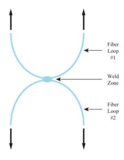
Figure 8: Schematic of weld strength test.
