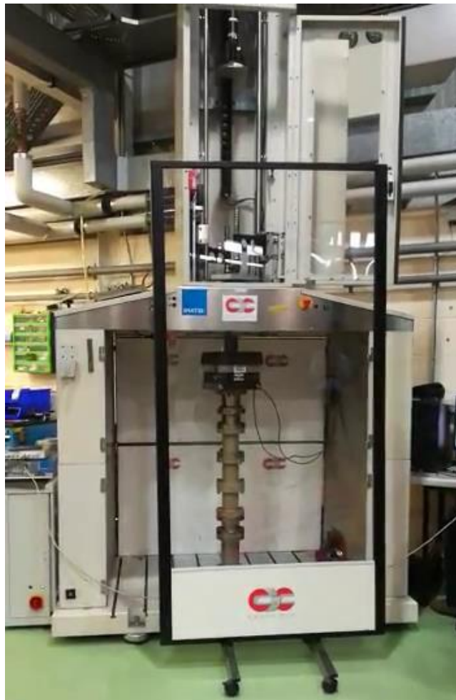
Figure 4-1. CIC's drop tower rig used for the physical testing of the specimens
