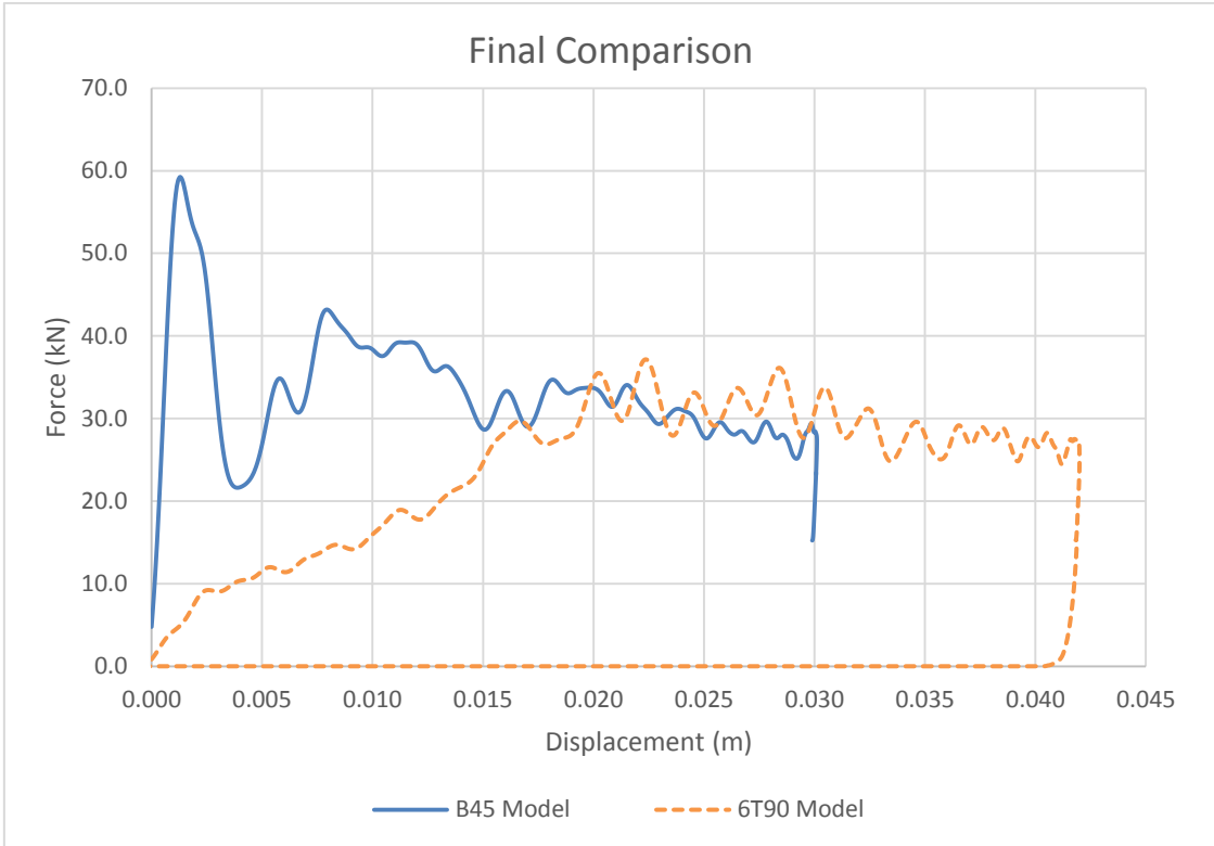
Figure 7-15. Final comparison of the best bevel and tulip triggers found.
