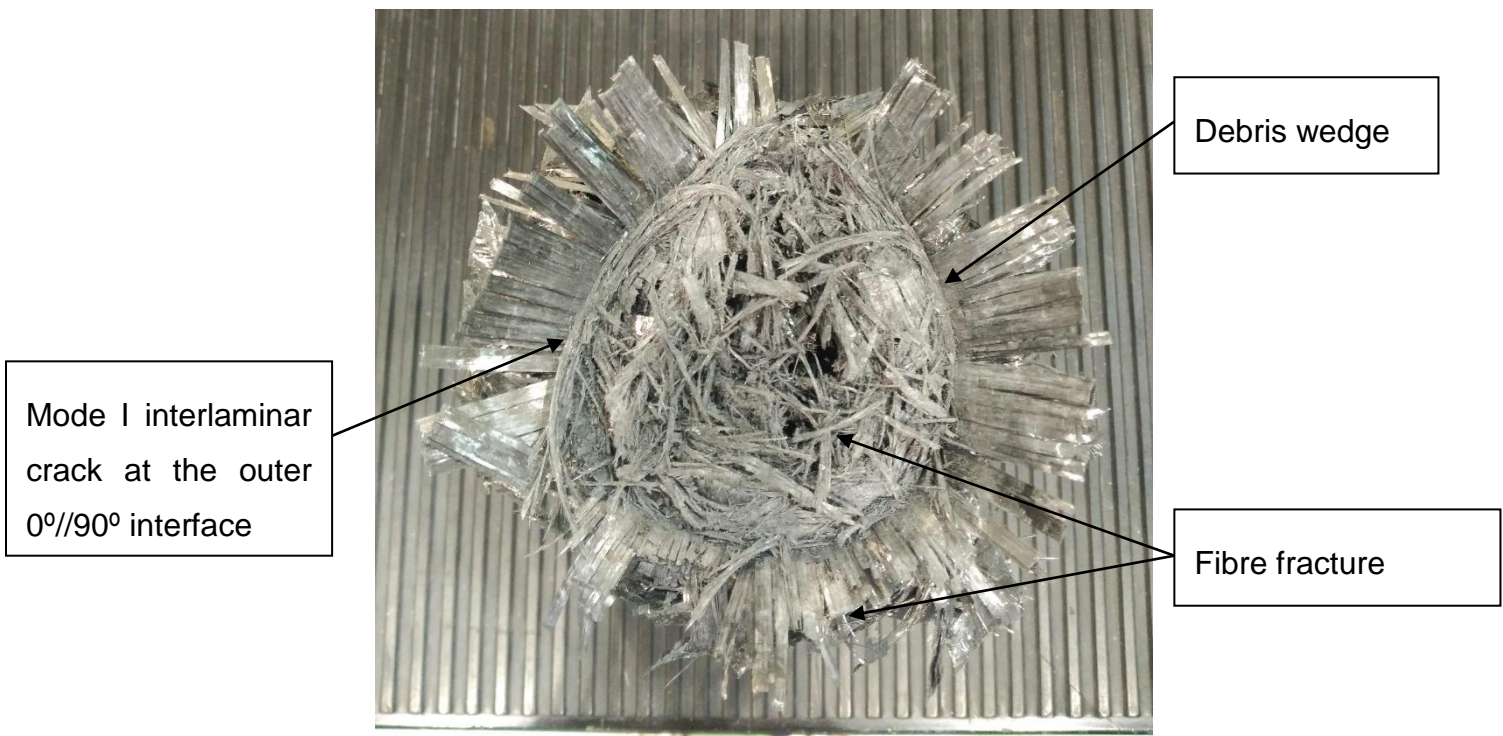
Figure 5-2. B60 specimen after impact testing. Top view.
