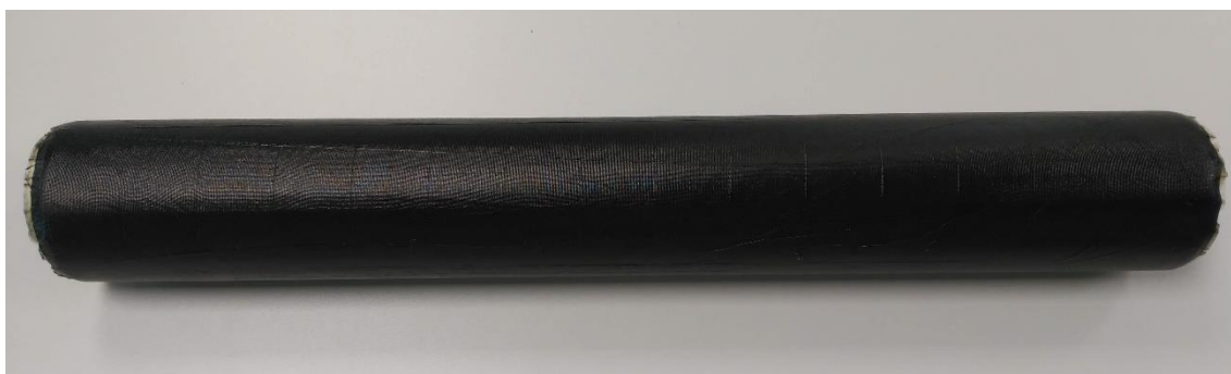
Figure 3-9. Cured tube released from the mould
