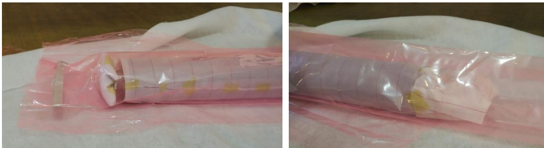
Figure 3-5. Tube covered with the peel ply material.
