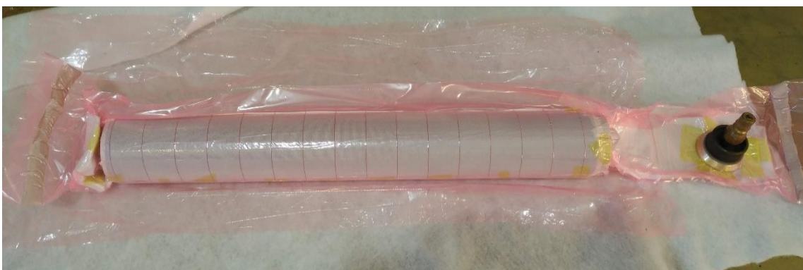
Figure 3-7. Tube setup for the curing process.
