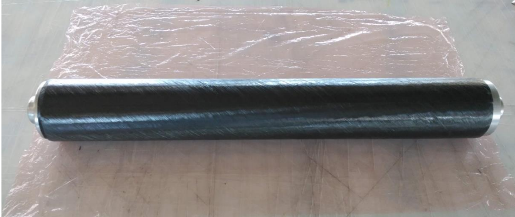
Figure 3-4. Tube after the laminating process.
