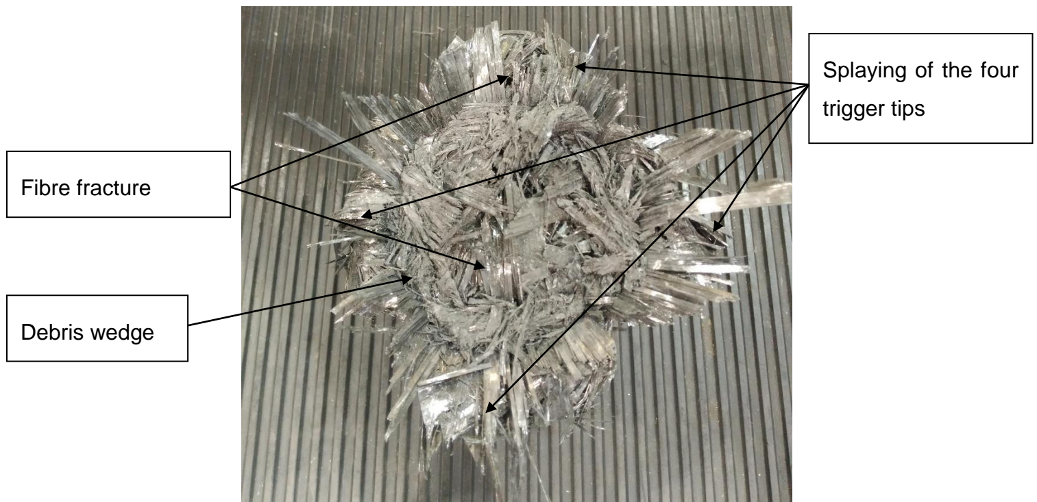
Figure 5-7. 4T60 specimen after impact testing. Top view.
