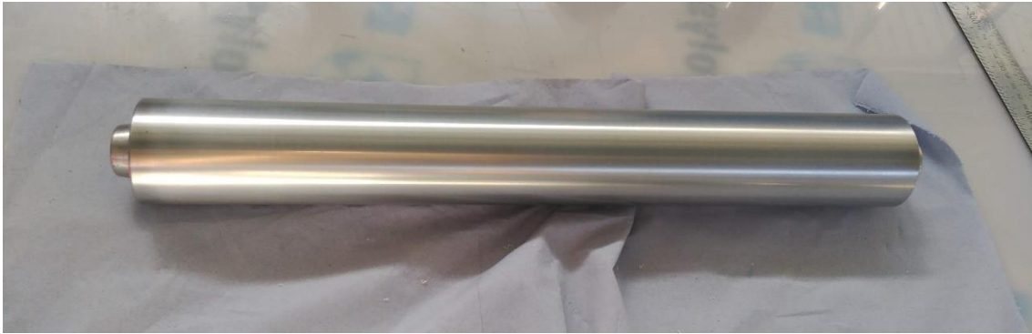
Figure 3-1. Metallic mandrel used as a mould for the tube's manufacturing.
