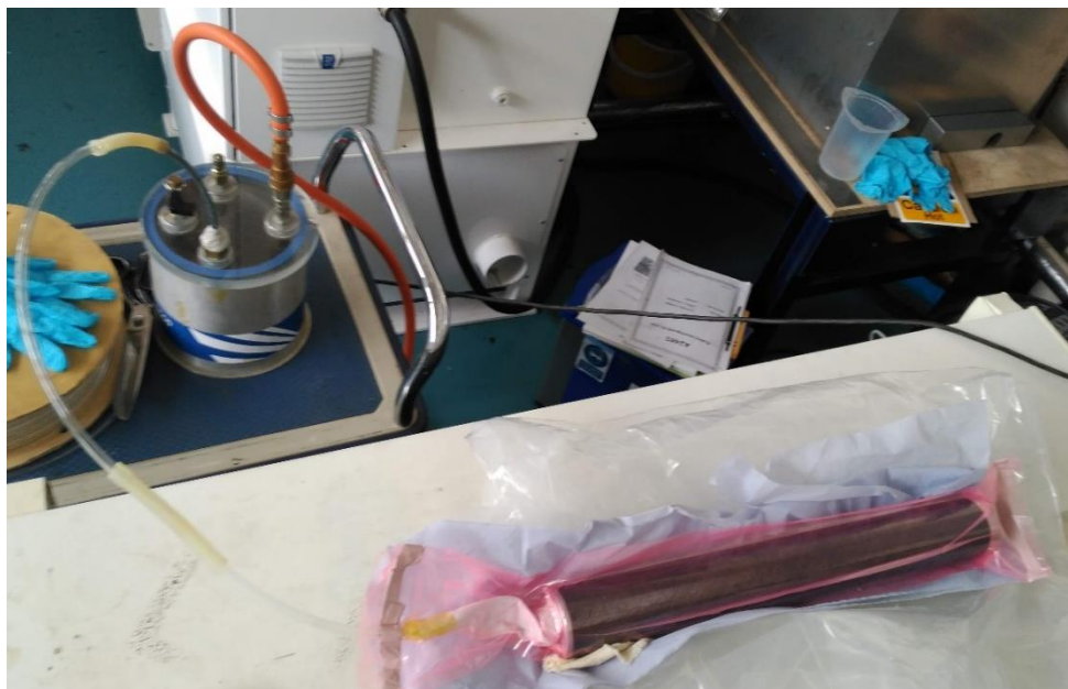
Figure 3-3. Debulking process set up.
