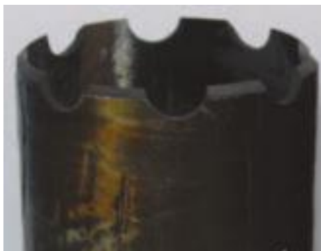
Figure 2-11. Detail of the crown trigger suggested by Huang [31]. (Adapted from Huang [31]).
