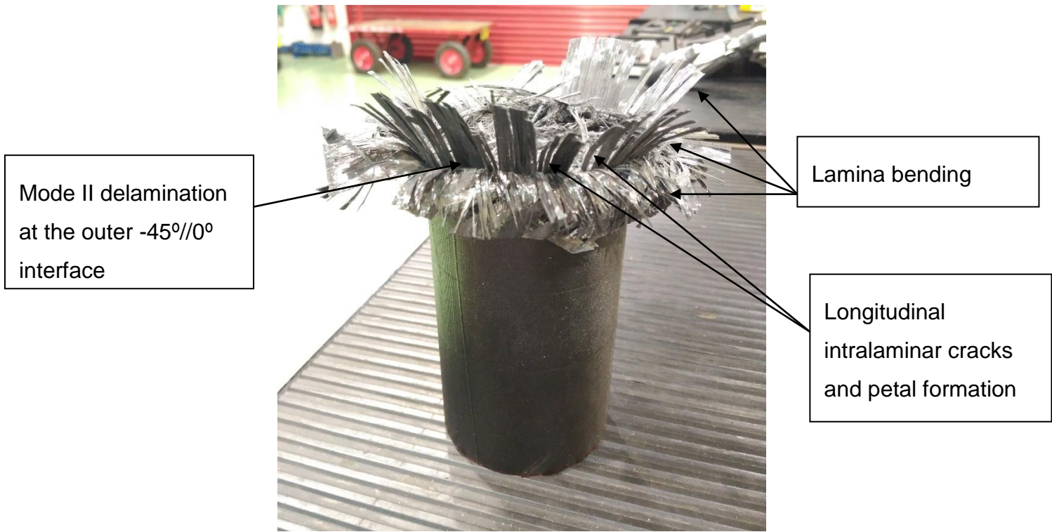
Figure 5-1. B60 specimen after impact testing. Overview.
