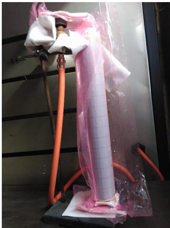
Figure 3-8. View of the oven's interior with the tube set up for curing.
