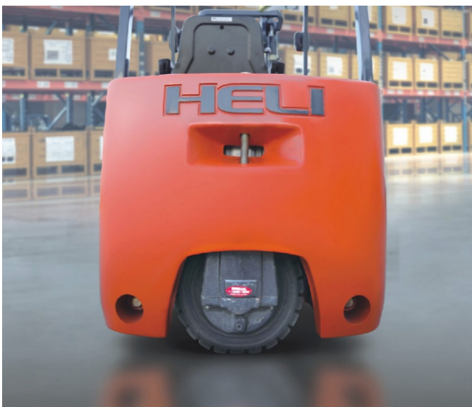
Example of a rear drive wheel motor, with the rear wheel totally turned. (Heli)
