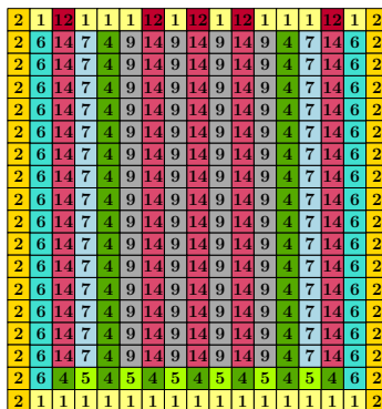
Figure B.6: Axial definition of the NEACRP reactor.
