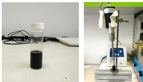
Figure 3.3. Ink (left) and ultrasonic mixed (right).
