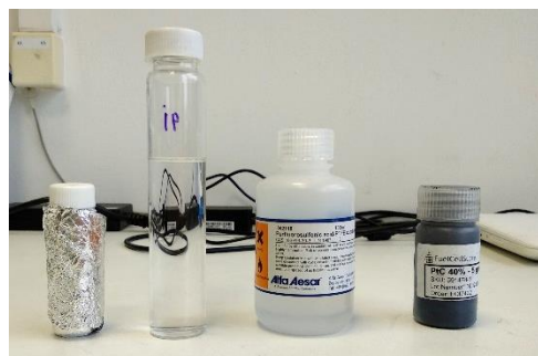
Figure 3.2. Ink compounds. Left to right: teflon, isopropanol, nafion, catalyst powder.
