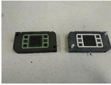
Figure 3.5. At right it is seen one graphite plate and left, MEA on top of the other graphite plate. On green and white the gaskets.
