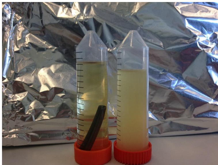
Figure 2.18: Qualitative measurement of the specimen's turbidity compared with the positive control.
