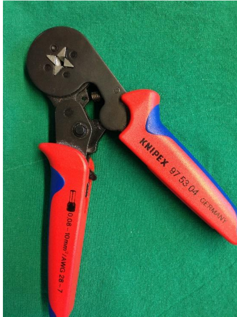
Figure 2.15: Self-adjusting crimping pliers used for the closing of one of the tube ends.
