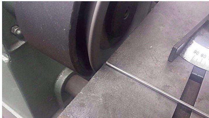
Figure 2.14: PCD finishing process with the grinding machine.
