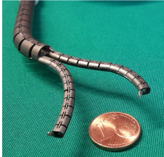
Figure 2.7: Functional prototype of the Double Arm Endoscopic Mini-Manipulator System (MiMed) based on compliant mechanisms in its overtube, as well as in its both arms.
