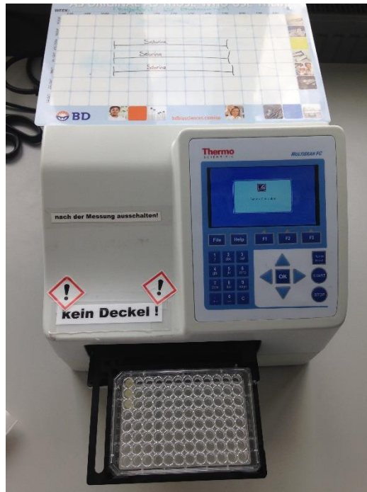
Figure 2.19: Spectrophotometer with a 96-well plate containing 100 \mu l swabs of each PCD.
