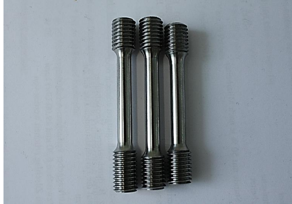
Figure 2.10: Dog bone tension test specimens.
