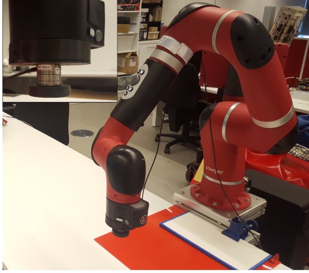
Fig. 1. Experimental setup: 7R serial manipulator with a force sensor rigidly attached to the robot end-effector, a tool consisting of a cylinder of 43x43x10mm attached to the sensor to emulate a tool and an object with flat flexible surface as target.
