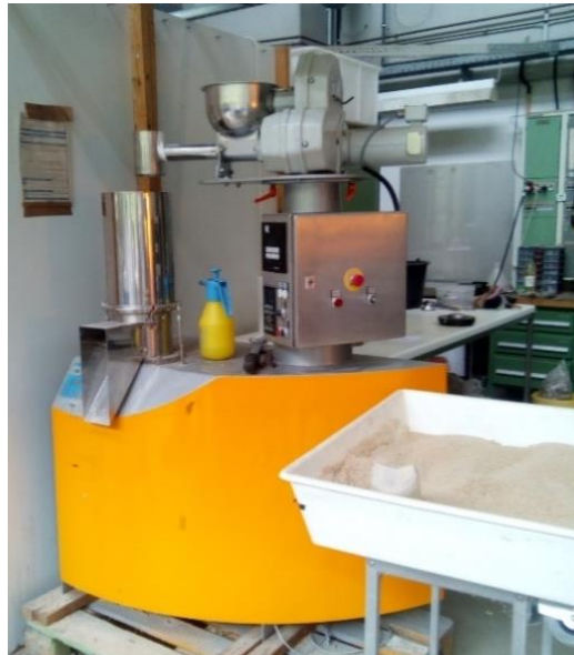
Figure 12. Pelletizing press model 14-175.
