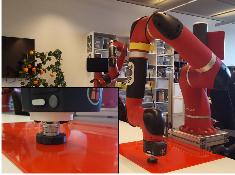
Figure 5. Experimental setup: 7R serial manipulator with a force sensor rigidly attached to the robot end-effector, a tool consisting of a cylinder of 43x43x10mm attached to the sensor to emulate a surface preparation operation and a flat surface as target.
