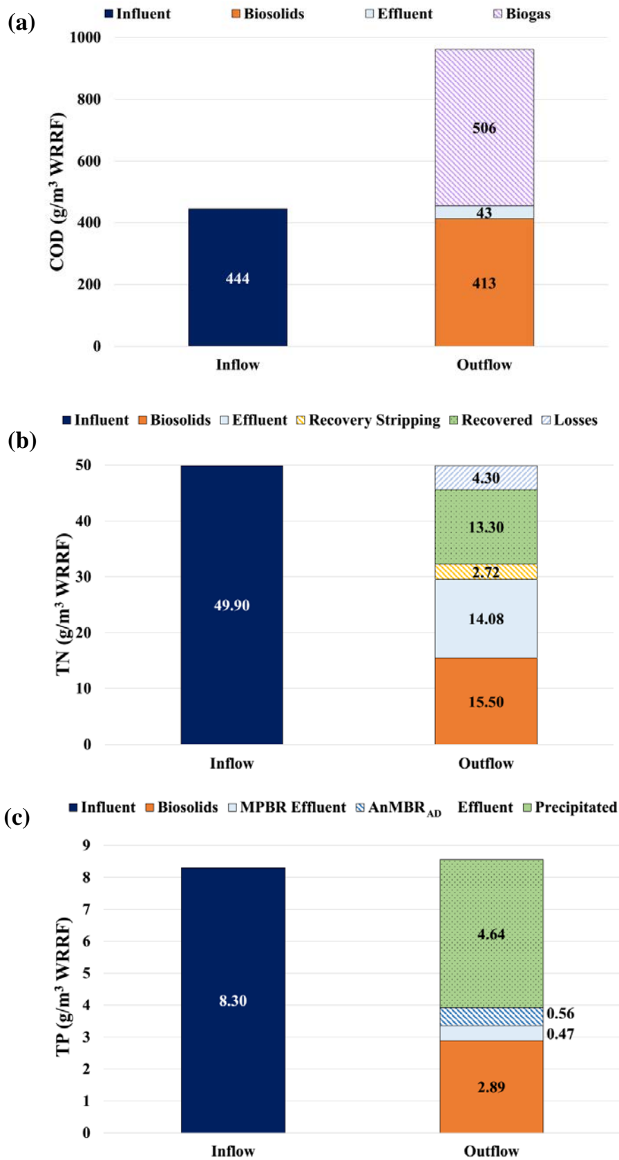
2 Figure 2: WRRF mass balances for: (a) COD, (b) TN and (c) TP.
