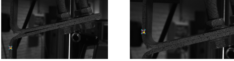
(a) Inferior plate DIC detection zone (b) Superior plate DIC detection zone
