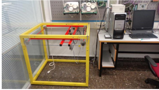
Figure 5. Cartesian robot (3D CRANE module).
