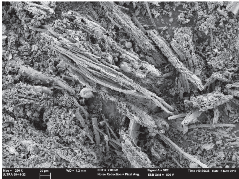
Fig. 2. SEM-ES micrograph of SCBA calcined at 600°C in an electric oven for one hour (EO600)
