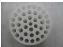
Figure 2.2 Multidrilled Teflon® mold used to fabricate 3D structures of hyaluronan.
