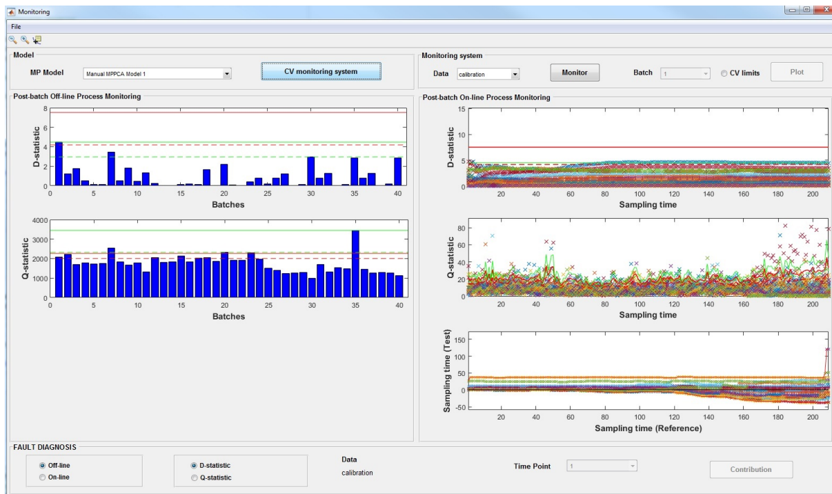
Figure 8: Interface for the design of a monitoring scheme and the monitoring of test batches.
