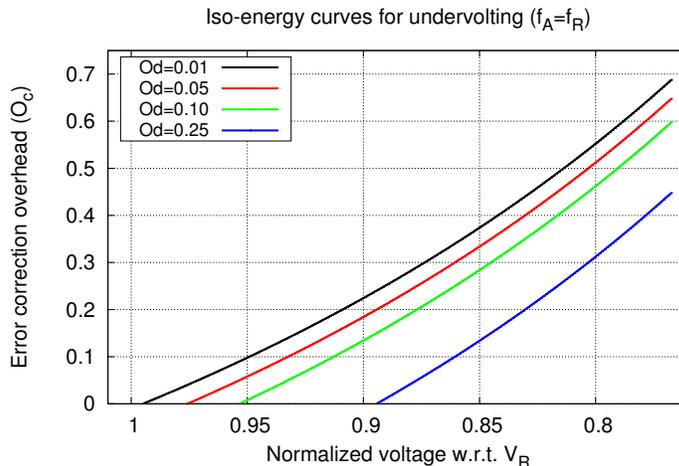
Figure 3: Configurations for the fault-tolerant versions of DLA operations, operating in undervolting conditions in the Cortex-A15, that attain the same energy efficiency as the original routines executed in the reference configuration  $C_3$  without errors.
