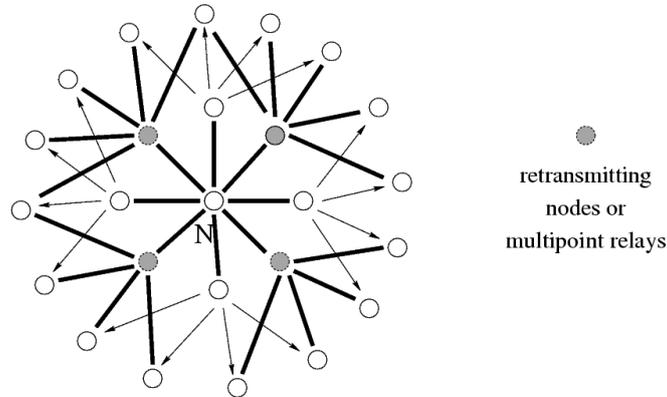
Figure 4.3: Illustration of the multipoint relay concept for node N.
