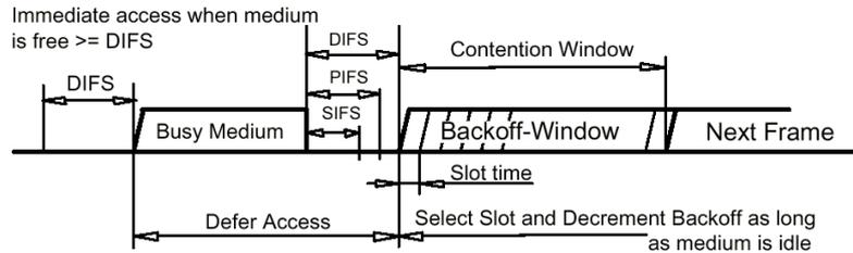
Figure 3.6: The CSMA/CA mechanism.
