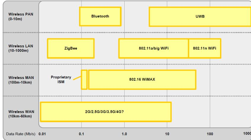
Figure 3.1: Bandwidth variation with range for different wireless technologies.
