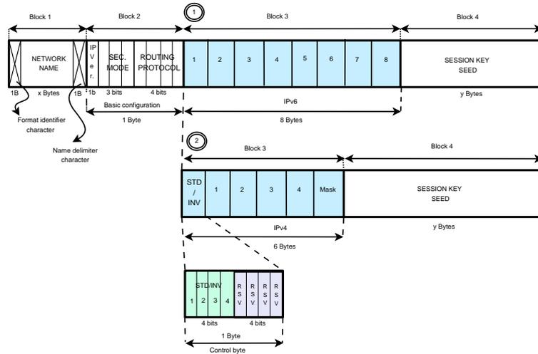
Figure 6.12: Detailed SSID partitioning strategy.
