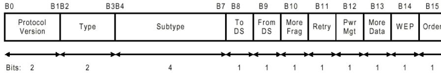
Figure 3.5: Information contained in the frame control field.
