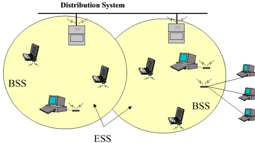
Figure 3.7: Example of a distribution ESS aggregating two BSSs.
