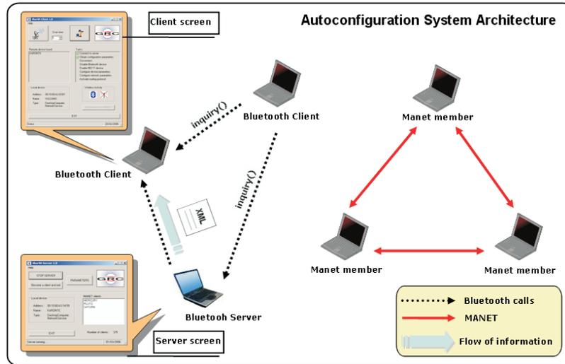
Figure 6.1: System architecture.
