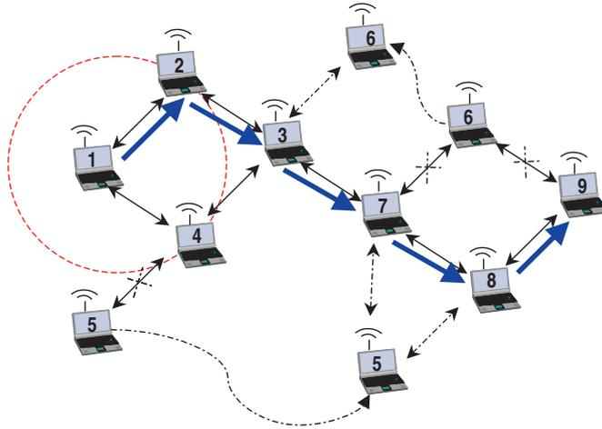
Figure 4.2: Example of multi-hop routing in MANETs.
