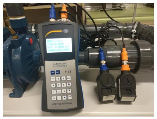
Figure 2. Ultrasound flow meter
