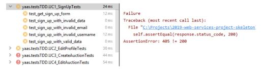
Figure 3. Example of failed tests.
