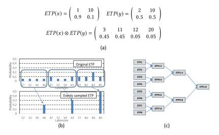
Figure 5: SPTA basic concepts: (a) convolution; (b) sampling; (c) inter-ETP parallelization.
